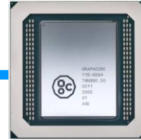
Graphcore - GC200 IPU AI chip, 7 nm 1,472 cores 59.4 Billion Transistors
